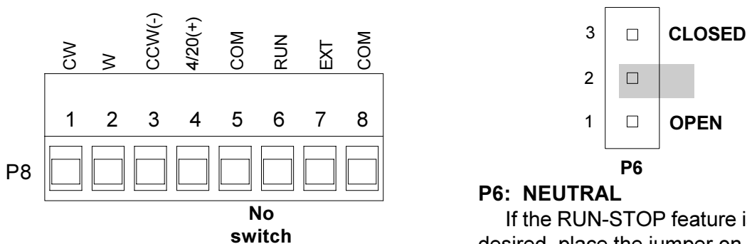
Figure 6. Disabling the external run-stop switch feature.
