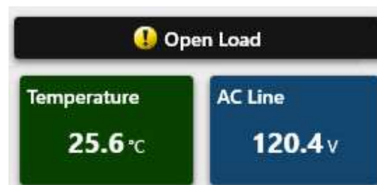
Example Control Panel Dashboard showing an Open Load Warning Alarm
