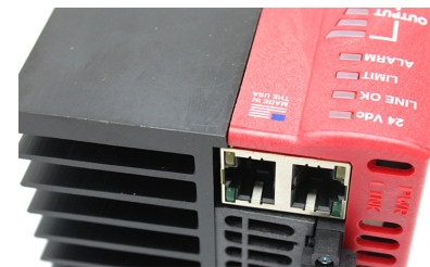
Figure 10.00: Side view of a MicroFUSION to show location of LEDs.
